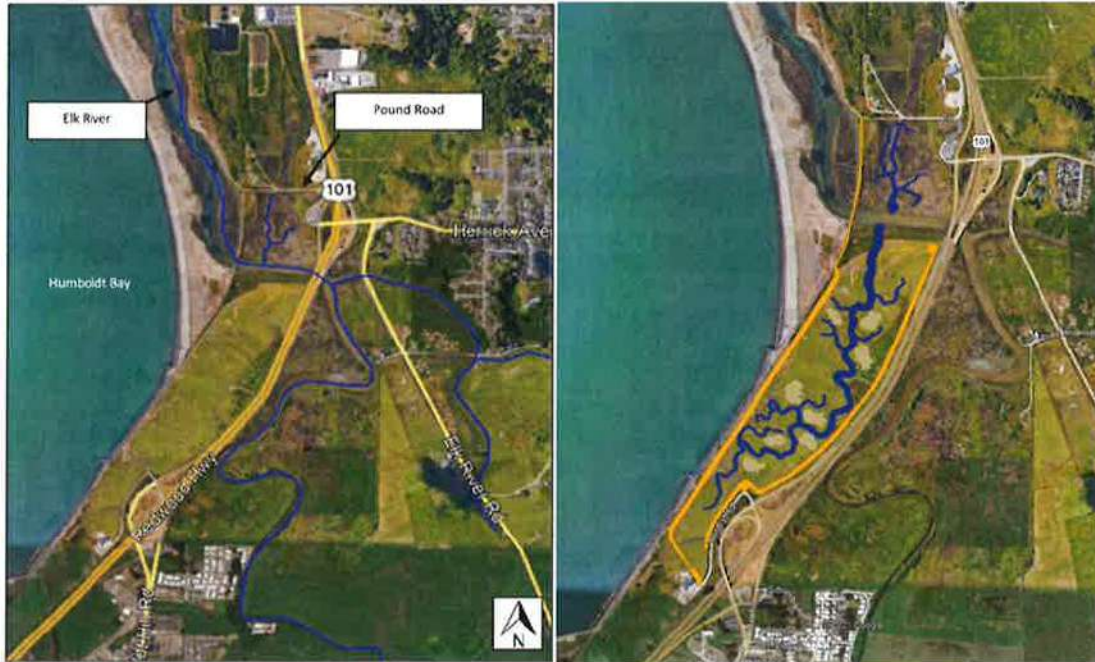
Figure 8: Site Images Showing Existing Channel North of the Elk River in 25 Acres of Area 1, and Existing Pasture South of Elk River in 89 acres of Area 2. Proposed Channel Network in Blue and Tidal Ridge in Yellow.
