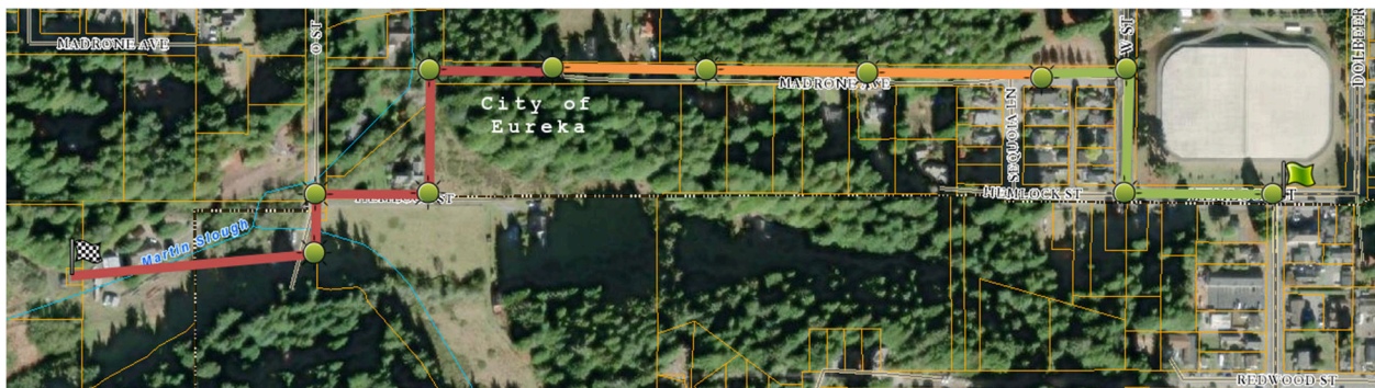
Figure 1: A depiction of the Hemlock Sewer Reversal project extending from the intersection of Walnut and Hemlock (green flag) to the O Street station on the Martin Slough Interceptor (checker flag).
