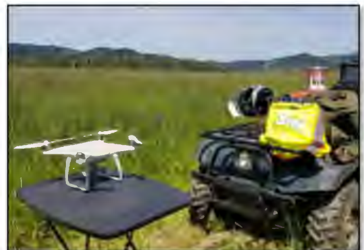
SHN's UAV equipment includes multi-rotor vehicles, as pictured above. The spatial accuracy, high resolution, and surface modeling obtained from processing UAV data is a powerful asset for survey services.
